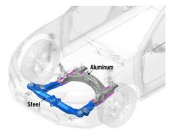
FSW of Aluminium and Steel on Honda Accord front subframe from 2013 (www.honda.com)
